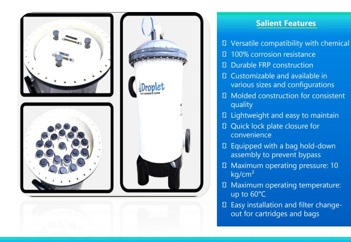
This Multi Cartridge Filter Housing is especially beneficial for applications that demand high flow rates in confined spaces, efficiently processing large volumes of water in a compact design. The use of FRP material ensures durability and reliability in harsh environments where metal housings may be prone to corrosion or deterioration.
